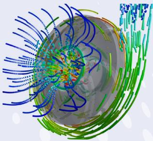
3D simulation software enabled Hendor to optimize internal pump geometries resulting in significant increases in pump efficiencies with improvements up to 30% versus the previous D170 series. The new D18 vertical pump range based on this innovation allows the surface finishing industry to reduce the life cycle cost of their pump base significantly.
